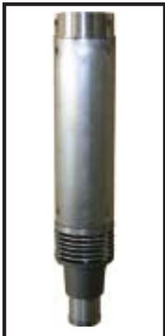
The extended diffuser is a drop tube extension with a Morrison Diffuser attached. If the tube is too short to meet code, purchase the extended diffuser instead of replacing the tube. This diffuser provides an additional 12" of length to the drop tube.
