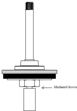
We are recommending that you replace any old style plungers, found during valve maintenance, with a new complete plunger. The part numbers and list prices for these new assembled plungers are:
