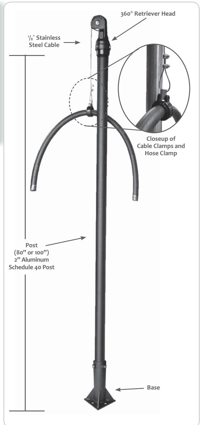
11. If you want to adjust the cable length, or for any reason you need to remove the cable clamps, see Figure 1 below before reattaching clamps.
