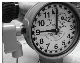
Figure 5: Hold thumb nut at desired trip point. Example - Alarm set point at 9 feet-0 inches.
