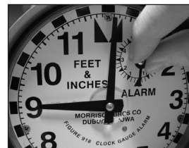
Figure 6: Setting Alarm pointer. Example - Alarm will now sound when level reaches 9 feet - 0 inches.
