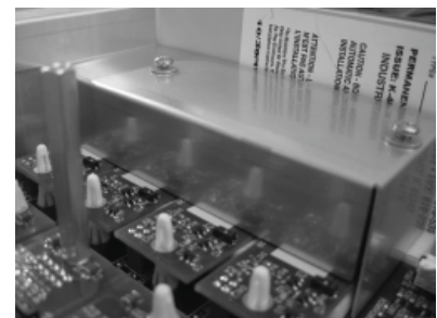
Figure 7 - Installing the I.S. cover
