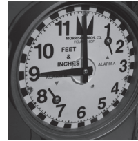
FIGURE 5: Hold thumb nut at desired trip point. Example- Alarm set point at 9 feet - 0 inches.
