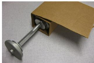
4. Next locate the poppets inside the cardboard insert. See right photo above. Place a gasket on each of the poppets (the gaskets are both the same and will fit either poppet). Gaskets should be free of any foreign particles such as cardboard dust. Wipe clean if necessary.
